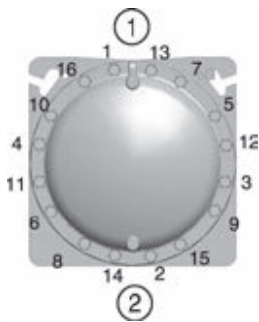
Water box tightening sequence
